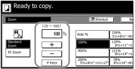
**2** Press [+] and [–] to set the displayed magnification. Press [# keys] ([#-Keys]) to enter with numeric keys.
